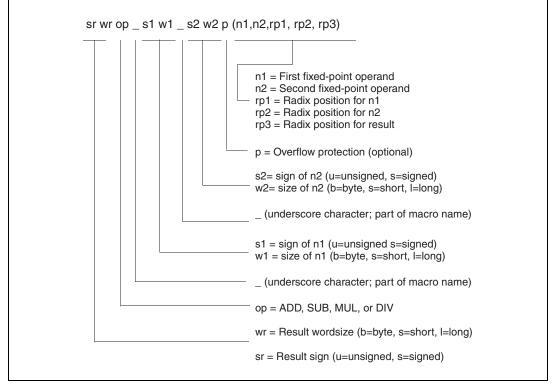
Figure 2-9. AutoCode/C Arithmetic Macros
